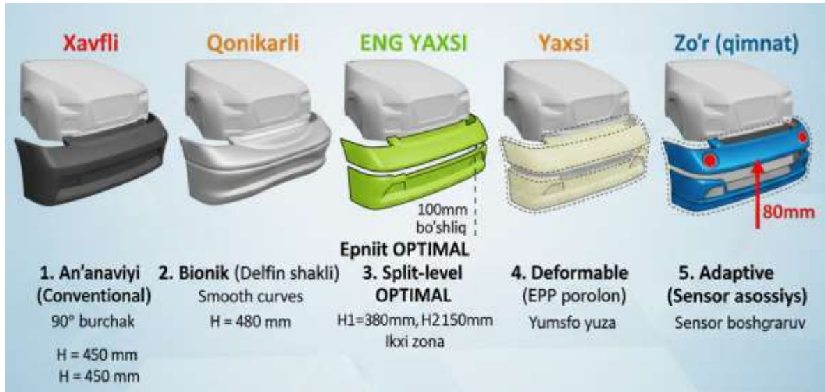
2-rasm. Besh bamper geometriyasining virtual crash test taqqoslashi
