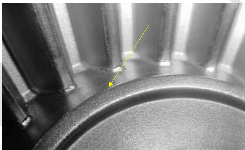
2-rasm. Konussimon shesternyani shtamplash uchun mo'ljallangan shtampning 400 sikldan so'ng buzilishi [1]
